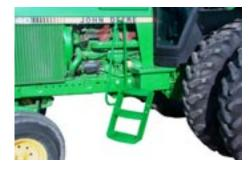
When attaching steps and hand holds, steps should be welded or bolted to the tractor frame or existing steps. Steps should be made of steel with non-skid, non-slip tread materials.
