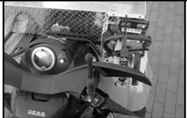
A modified ATV with a storage box and chainsaw mount. This one is constructed out of diamond plate instead of wood.
