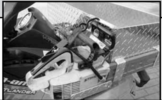
A modified ATV with a storage box and chainsaw mount. This one is constructed out of diamond plate instead of wood.
